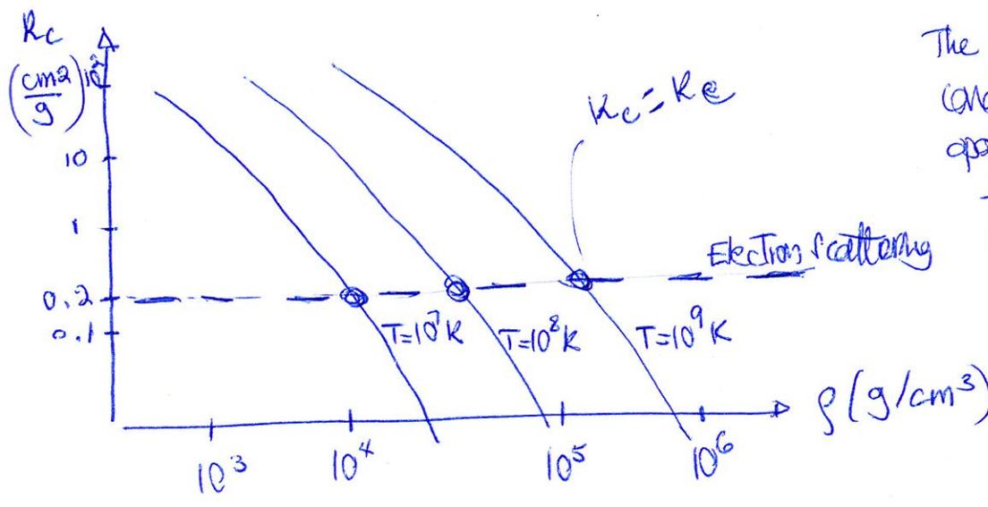
The density at which the conductive opacity = radiative opacity due to scattering from the electrons increases ~ one order of magnitude for each order-of-magnitude increase in the temperature.
