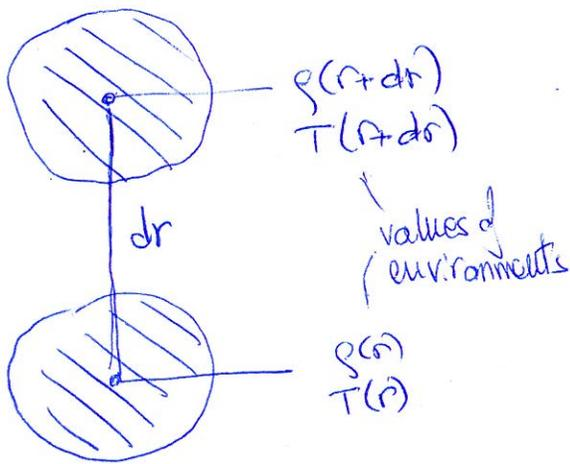
The mass element is displaced by  $dr$  without exchanging heat with the environment (i.e. adiabatic change)
