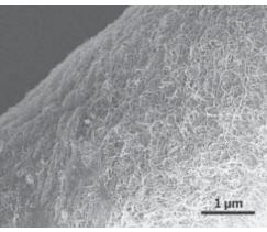
**FUNCTIONAL** The spider silk fibers shown in these SEM images were coated with gold (top) and carbon nanotubes (bottom) to render the micrometer-sized threads conductive and useful for electronics applications.
