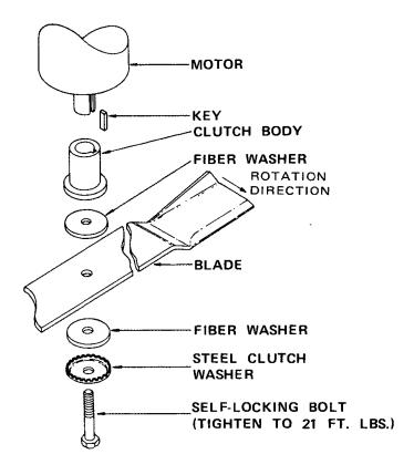
If reusing an existing key, ensure that edges are square and sides are flat. Replace if needed.
